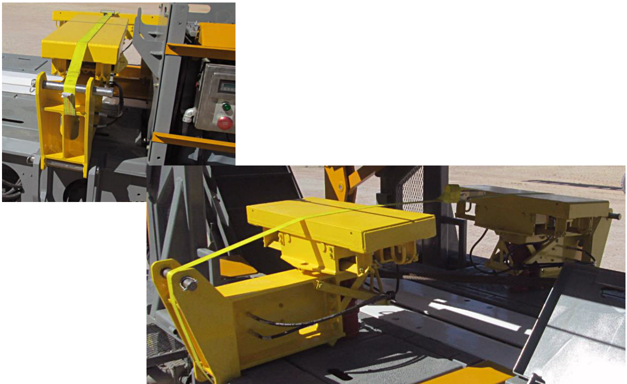
Figure 3: Pad walkers properly strapped for transport
