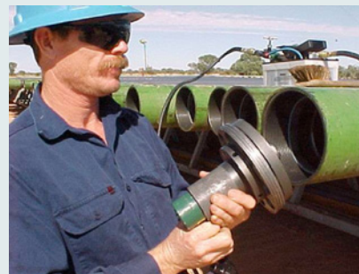
Installation is fast and easy with a simple handheld hydraulically actuated tool. Rings can be installed in the field, pipe yard, and/or pipe mill.
