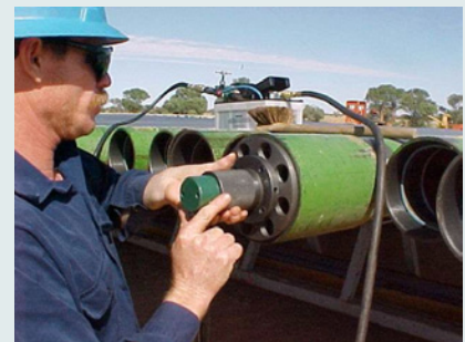
Installation is fast and easy with a simple handheld hydraulically actuated tool. Rings can be installed in the field, pipe yard, and/or pipe mill.
