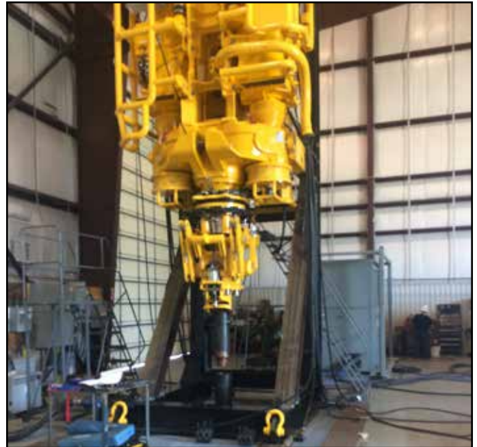
An HPS 1000 top drive is tested in Tesco's dynamometer.
