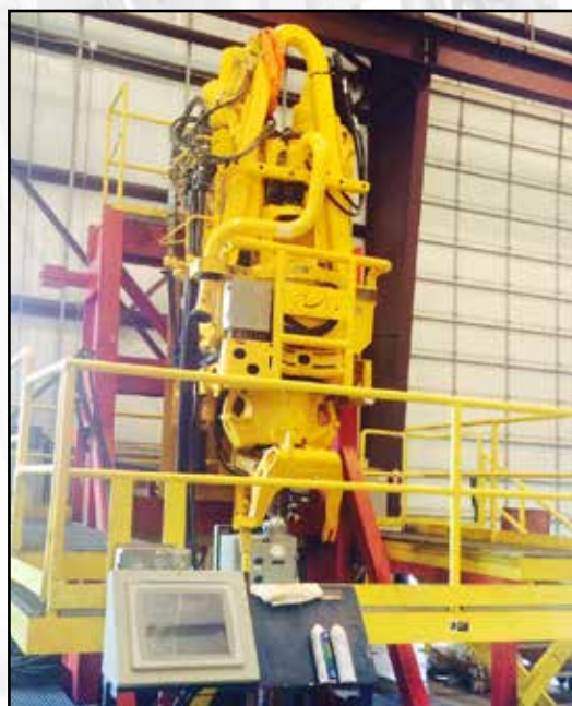
Tesco dynamometer tests an NOV TDS-11 Top Drive
