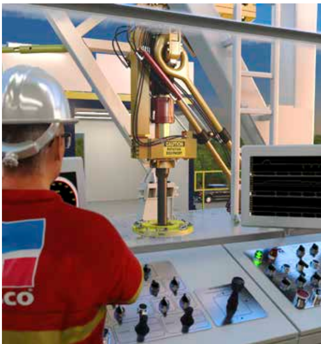
Figure 2. ARC software uses well plan details and live rig data to accurately model drill string characteristics and adjust top drive parameters in real time to enhance and optimise the drilling process.
